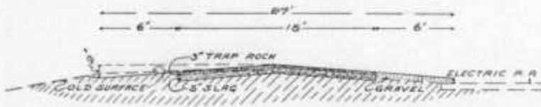
FIG. 14.—Typical cross-section of Eastern avenue, Baltimore county, showing macadam construction with slag foundation and trap-rock top course.
