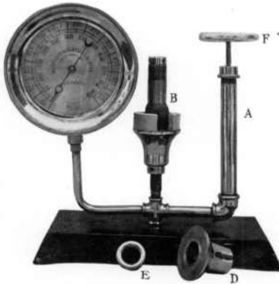
FIG. 2.—MACHINE AFTER A TEST WITH THE TOP CAP REMOVED, SHOWING THE BROKEN CEMENT RING AND DISTENDED RUBBER CYLINDER OR TUBE.
