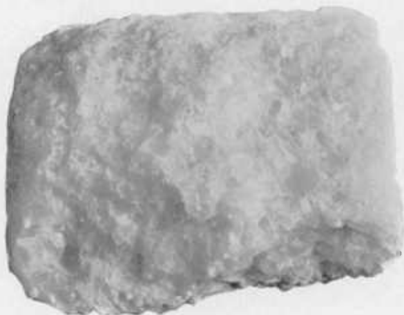
FIG. 1.—“ALUM STONE,” DITMAN QUARRY, TEXAS. WHITE CRYSTALLINE MARBLE COMPOSED OF LARGE CRYSTALS OF CALCITE.
