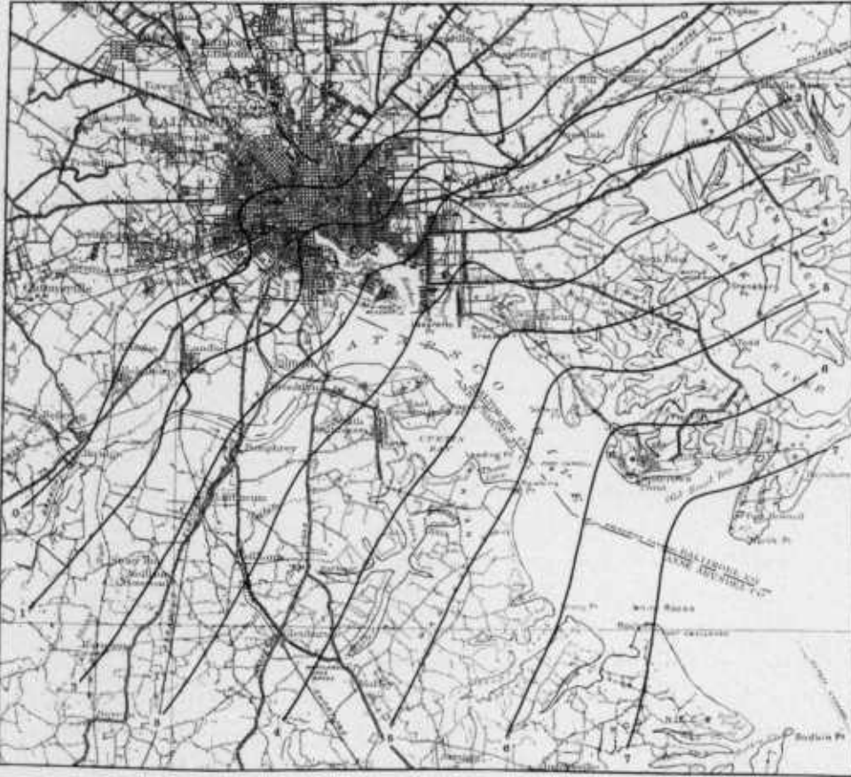
FIG. 90.—MAP OF THE BALTIMORE DISTRICT. CONTOURS AT 100-FOOT INTERVALS SHOW THE APPROXIMATE SURFACE OF THE UNDERLYING CRYSTALLINE ROCKS FROM WHERE THEY PASS BELOW TIDE (0) DOWN TO 700 FEET.
