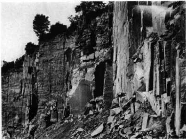
FIG. 1.—Longitudinal joints facing reader, regional tension joints and cross joints normal to them in the Port Deposit quarry.
