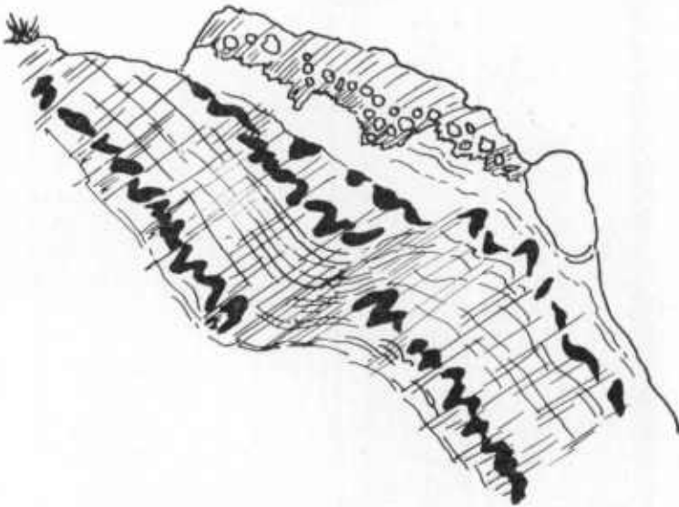
FIG. 9.—Bedding in Conestoga limestone almost obliterated by slippage along cleavage planes. Burnt Mills, Pennsylvania. Height of the exposure 10 feet.
