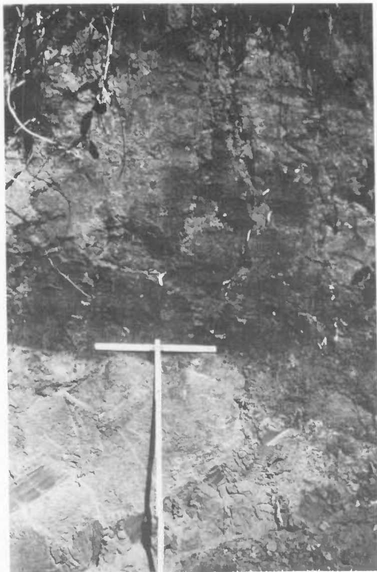
FIGURE 65: Contact between Hornerstown Formation and Monmouth Group (at crossbar of folding rule). Borings are present in both formations, as at the locality of figure 64, but do not show in this photograph. Rule is 2 ft (60 cm) long. North side of excavation during construction of Georgetown Post Office in Fredericktown. Contact is 5.5 ft above loading platform at rear of building.
